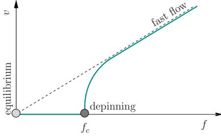
FIG. 2. (Color online) Velocity-force characteristics of an elastic manifold at  $T=0$ . The three self-affine reference states are: Equilibrium ( $f=0$ ); Depinning ( $f=f_c$ ); Fast flow ( $f \gg f_c$ ).
