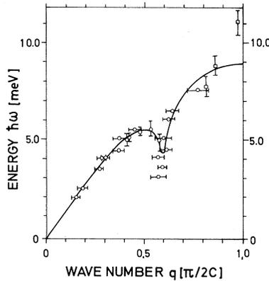
FIGURE 1 — *Kohn anomaly in the phonon spectrum of the quasi-1D conductor  $\text{K}_2\text{Pt}(\text{CN})_4\text{Br}_{0.3} \cdot 3\text{H}_2\text{O}$  at  $T = 300\text{K}$ . From : B. Renker et al, *Phys. Rev. Lett.* **30**, 1144 (1973).*
