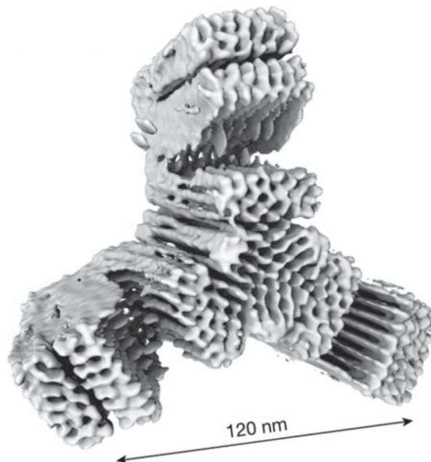
Example of a complex rigid structure manufactured using DNA origami (Wagenbauer, Nature 2017).
