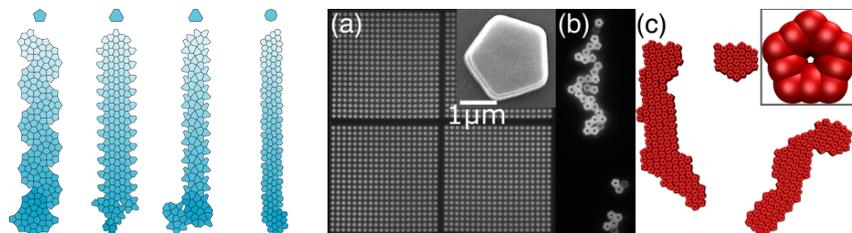
*Left: One-dimensional aggregates formed by identical particles (shown at the top) that cannot fit together to tile the plane unless deformed. Right: Our fluorescent 3D-printed particles (a) arranged in a regular array after printing and before detachment from the substrate and (b) after aggregation and their (c) numerical counterparts. Insets show individual particles.*
