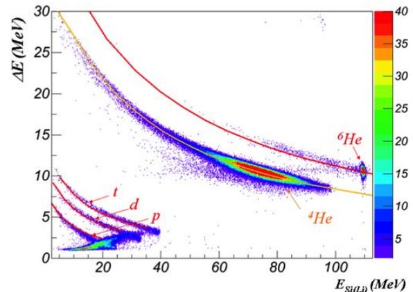
Fig. 4. Correlation between energy loss in the Si-strip detector versus energy loss in the Si-Li detector.  ${}^6\text{He}$ ,  $\alpha$ ,  $t$ ,  $d$ ,  $p$  can be identified.
