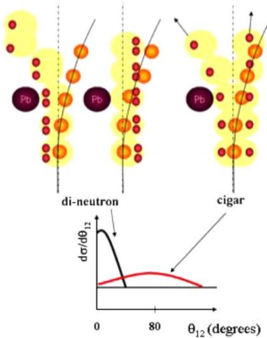
**Fig. 1.** Intuitive picture of the nuclear break-up of  ${}^6\text{He}$  in the di-neutron and the cigar configuration. When the two nucleons are close to each other, their relative angle after emission is small whereas it is large when they are on opposite sides with respect to the core.
