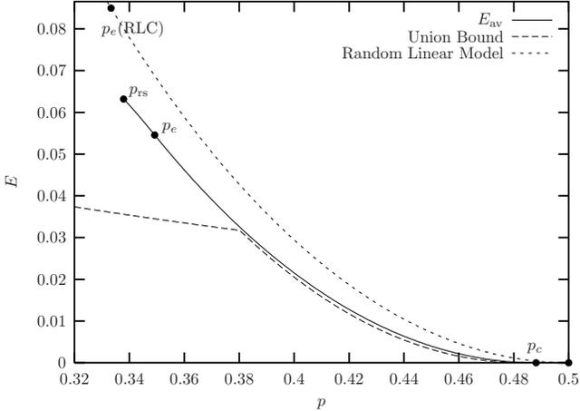
Figure 3: Average error exponent as a function of the noise level  $p$  of the BEC for the regular LDPC code ensemble with  $k = 6$  and  $\ell = 3$ . Gallager’s union bound and the random linear code limit (19) are also plotted for comparison.
