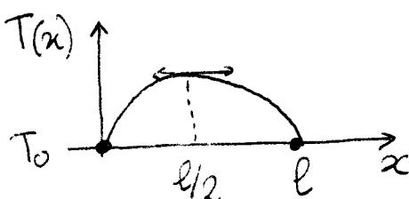
$$T_{\max} = T_0 + \frac{\sigma l^2}{8\lambda} = T_0 + 78K = 93^\circ C$$
