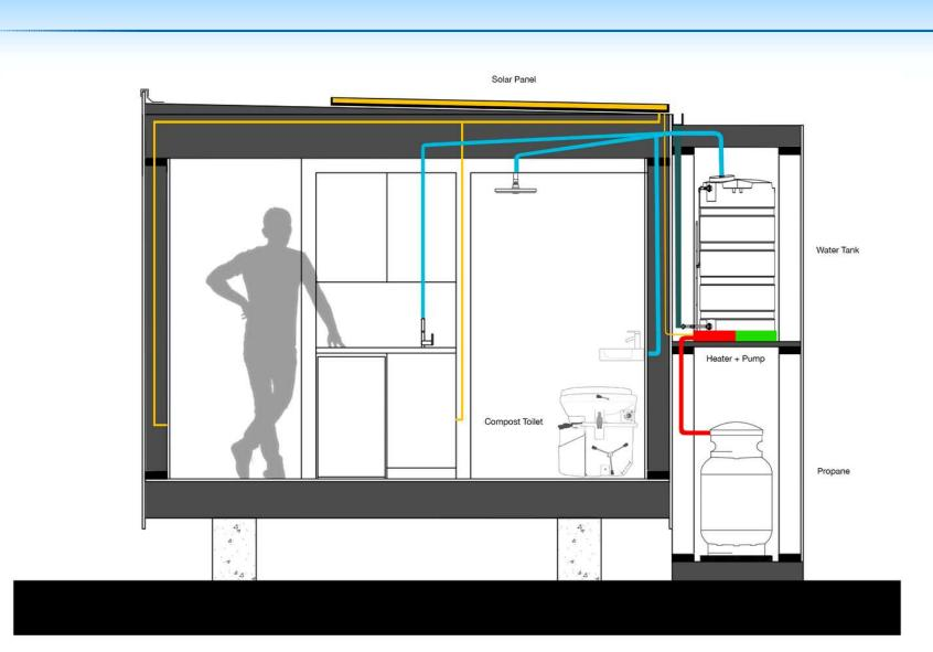
Edifice, Marc Thorpe Design, 2019 © Marco Petrini "All systems pertaining to the habitation of the cabin are "introverted" or traditionally defined as, "off-grid." These systems include solar power, water harvesting and composting toilet. Heating is provided by a wood burning stove and cooling is accomplished through cross ventilation. Lighting for the space is provided by candle."
