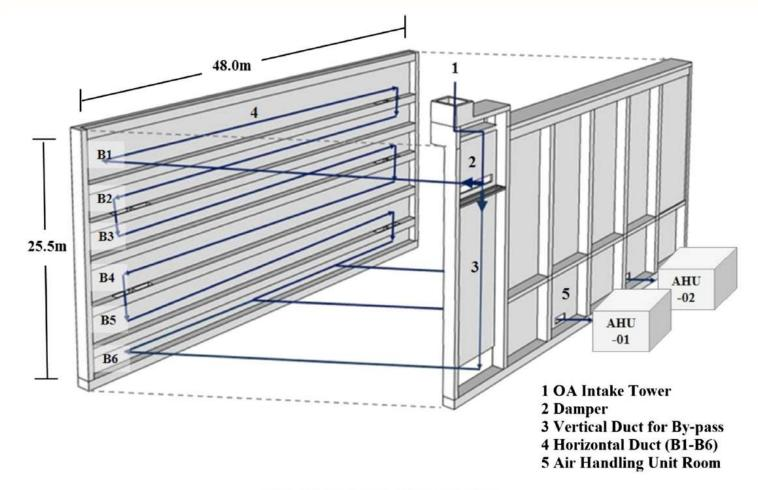
Fig. 4. OA intake channels of the measured TLVS.
