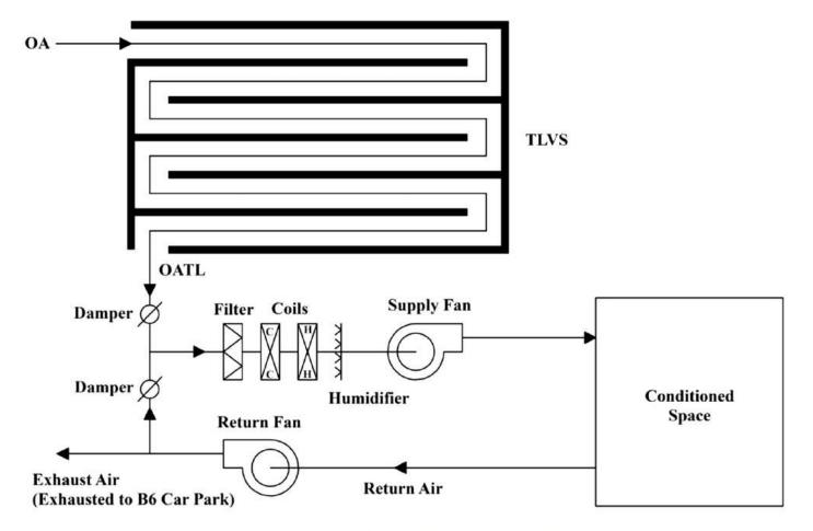
Fig. 5. Air flow diagram that includes the measured TLVS.
