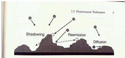
Fig. 1.3. Diagram of growth effects including diffusion, shadowing, and reemission that may affect surface morphology during thin film growth. The incident particle flux may arrive at the surface with a wide angular distribution depending on the deposition methods and parameters.
